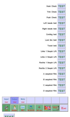
click the corresponding key of required testing items. check whether output has effect or not. if the output device no action. the output is fault. please check and repair.
